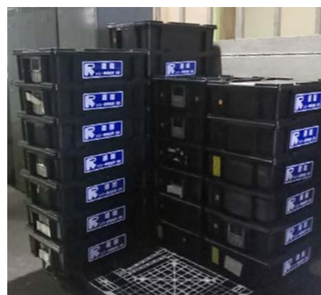
Returnable container used to transport components at Sony Global Manufacturing & Operations Corporation
