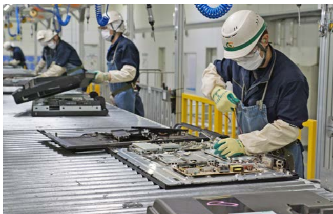
TV being dismantled at Green Cycle Corporation
