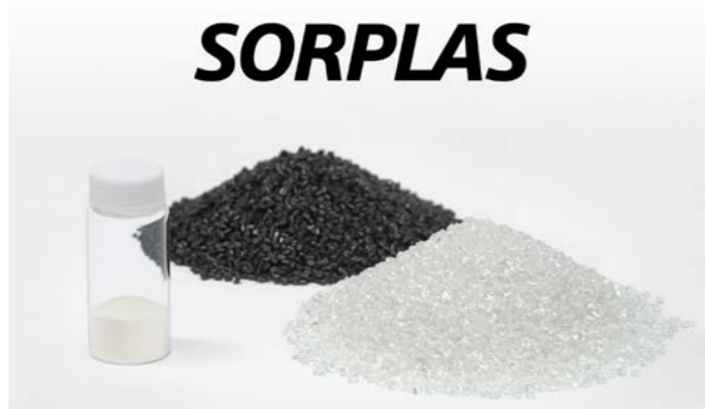
SORPLAS recycled plastic pellets (black), recovered pellets (transparent: right) and Sony's original flame retardant (left)
