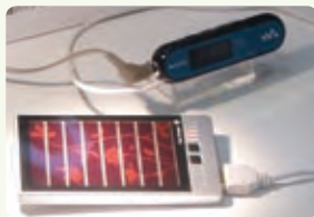
Demonstration of a prototype dye-sensitized solar cell/lithium ion battery hybrid charger being used to power a Walkman digital music player (December 2009)
