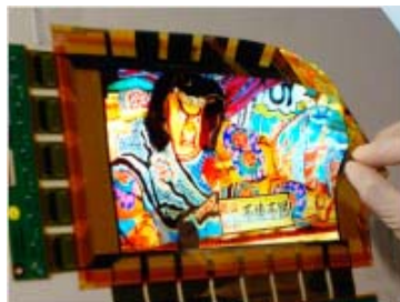
9.9-inch flexible OLED display prototype (June 2012)
