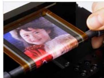
Organic TFT-driven OLED display prototype that can be rolled up (May 2010)
