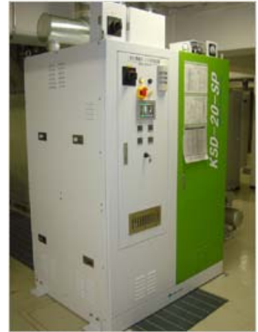
Small, fixed, condensing-type VOC treatment system developed by SCK in conjunction with an equipment manufacturer
