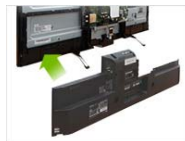
The 2013 Bravia™ W650A/W600A series snap-together structure required fewer screws.
