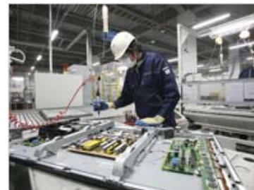
TV being dismantled at Green Cycle Corporation
