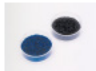
Polycarbonate resin for use in recycled shell casings
