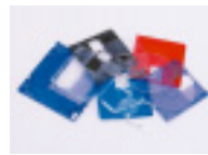
Waste polycarbonate resin produced from manufacturing processes
